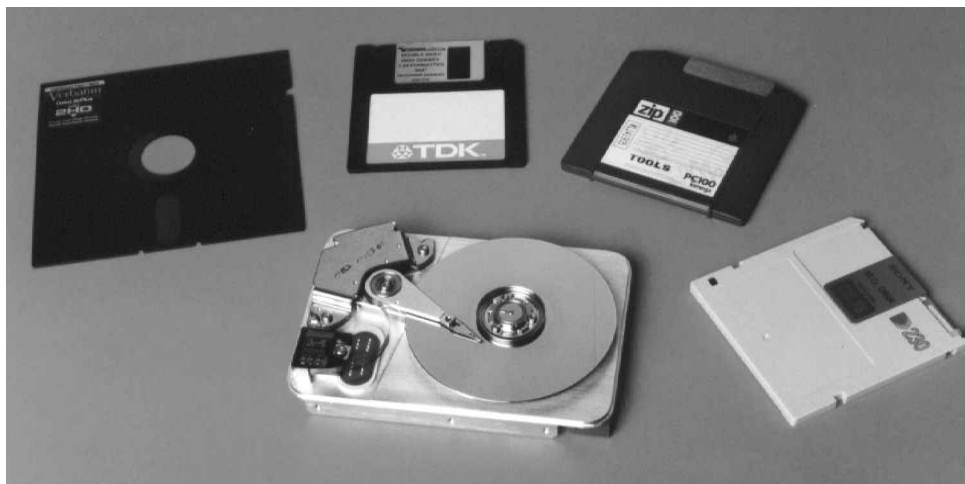
Figure 3. A survey of modern storage technology. From the left, an old 5.25'' floppy disk (100 kb), a modern 3.5'' disk (1.4 Mb), a Zip disk (100 Mb), a magneto-optical disk (up to 640 Mb). In the centre is an open hard-disk drive (up to 27 Gb).
